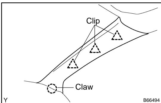
(b) Using a screwdriver, disengage the 3 clips and claw and remove the pillar garnish.
