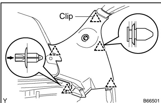
(c) Using a screwdriver, disengage the 5 clips and remove the side garnish.
